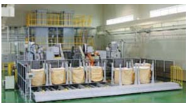
Solidification and automatic transport of scraps from cutting and grinding
