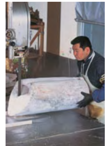
Metal Band Saw Blades for cutting frozen tuna
