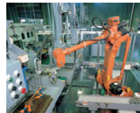
Loading Work for Machine Tools SC15F Layout that allows a robot to supply work for multiple machines Long hours of unmanned operation with Work Stocker
