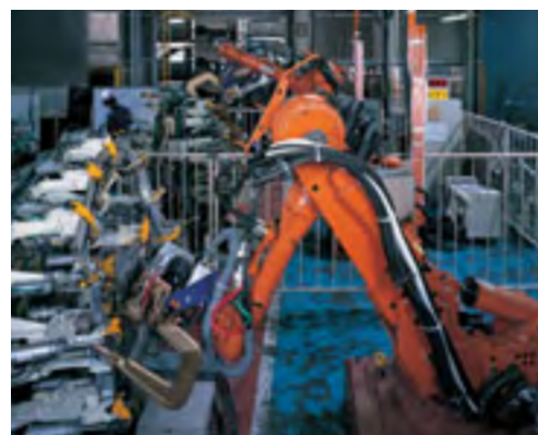
Spot Welding for Automobile Parts SH166 Making a factory clean and quiet with high-quality welding of no sputter
