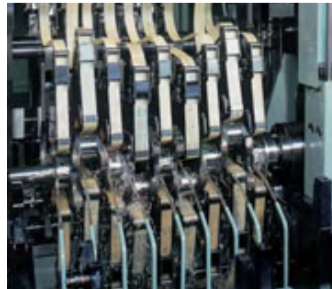
Improving surface roughness and roundness of crankshaft bearing surfaces.
