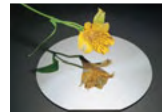
Surface of silicon wafer finished to have a mirror finish
