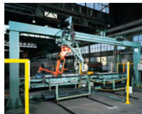
Arc Welding for Housing Materials SC15F Effective use of space with overhead suspension specification
