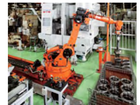
Material Handling with Vision Sensor ST166 Parts position detected by 3D Vision Sensing
