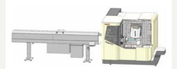
Multi-machining, cutting + gear-shaping, is possible with auto workpiece feeding (less than  $\phi$ 24).
