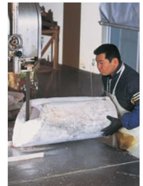
Metal Band Saw Blades for cutting frozen tuna
