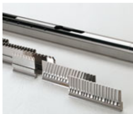
Broaches for Machining Compressor Vane Slots
