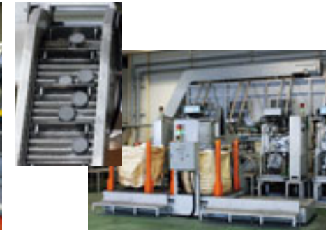
Metal sludge recycling system
