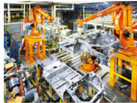
Spot Welding Robots Ultra-Heavy-Load Handling Robots
