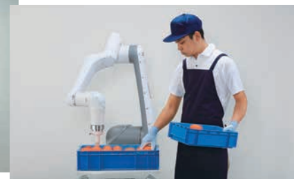
CZ10: human-friendly collaborative robot without a safety barrier
