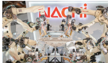
Spot welding robots (Used in the machining of EV bodies, etc.)
