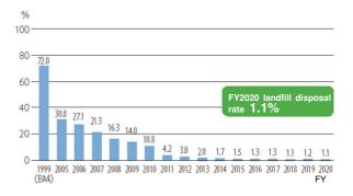
The landfill disposal rate\* is substantially reduced from 72.0% (BM) to 1.1% by recycling slag, expanding the use of waste liquid and sludge as fuels to generate power, Increasing the capacity of grinding sludge, and promoting its pressing to the extent possible. \* Definition: Landfill disposal rate = (Landfill disposal volume / Total waste generation volume) x 100
