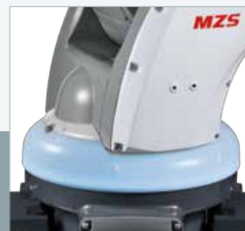
The stopper cover, which reduces the risk of getting pinched, has a built-in LED lamp that clearly indicates the robot's operating status with color, flashing, and a buzzer sound.
