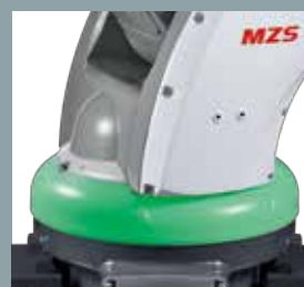
The stopper cover, which reduces the risk of getting pinched, has a built-in LED lamp that clearly indicates the robot's operating status with color, flashing, and a buzzer sound.
