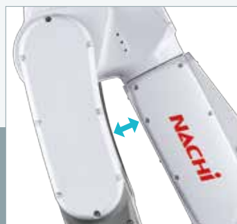
Offset arm shape for reducing clamping risk
