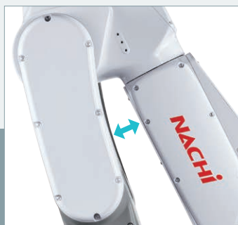
Offset arm shape for reducing clamping risk
