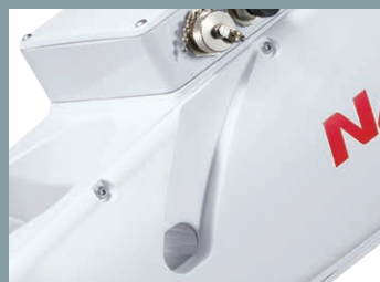
Newly designed cabling slit
