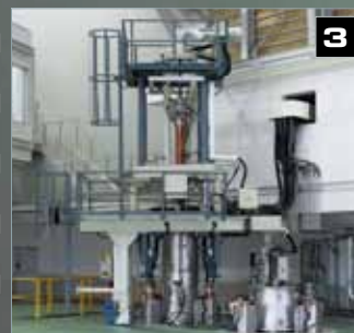
ESR furnace (electroslag remelting) 3 tons
