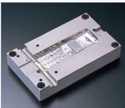
PROVA for molds for mobile phone casings Super-pure materials emphasize mirror finish and abrasion-resistance for molds for aspherical lenses and light guide plates.
