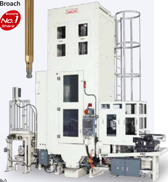
NC Helical Broaching Machine Performs highly efficient machining of helical gears for automatic transmission.
