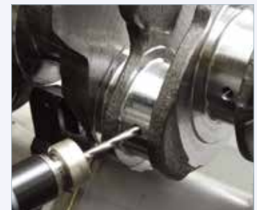
MQL Power Cell MQL Machining System High-efficiency, non step deep hole drilling.
